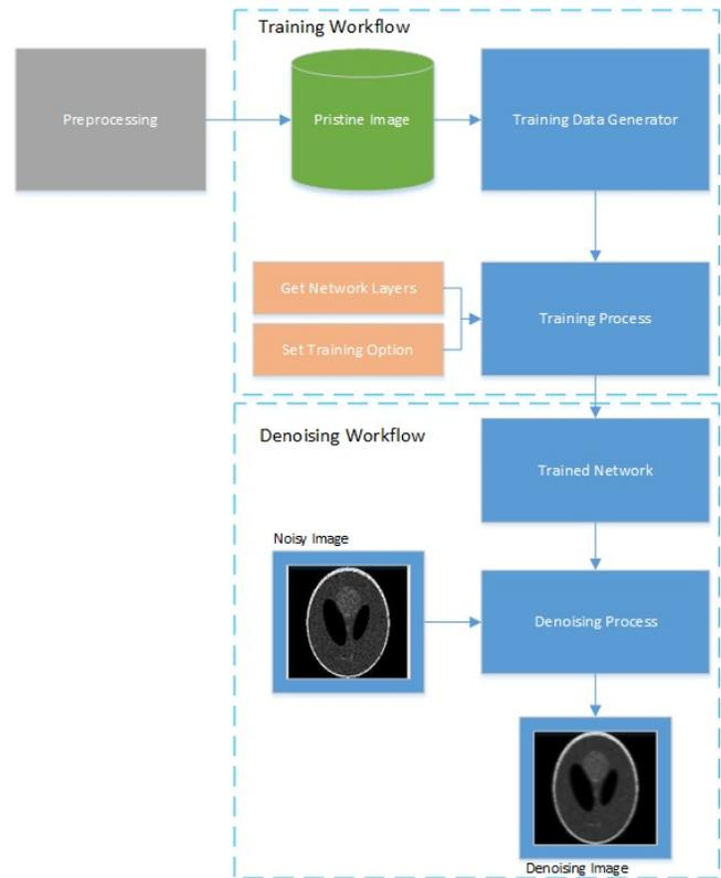
Figure 1: The proposed scheme for speckle noise reduction
