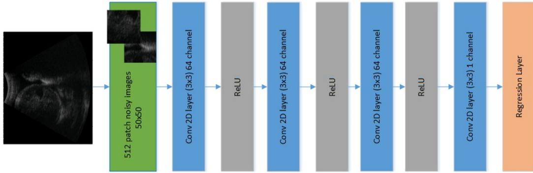
Figure 2: Simple denoising network layer
