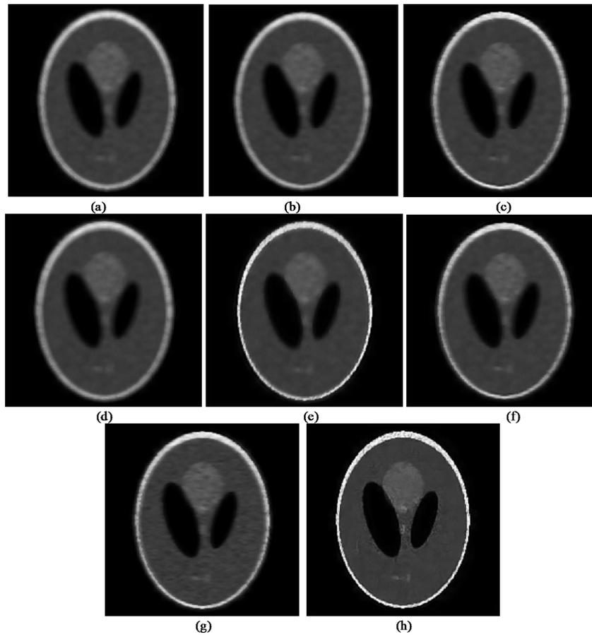
**Figure 3: Results of reducing noise using the method (a) Lee filter, (b) Frost filter, (c) bilateral filter, (d) dual-tree wavelet transform, (e) SRAD, (f) hybrid speckle noise, (g) 9-layer without preprocessing and (h) DnCNN model without preprocessing.**
