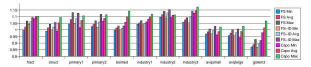
Figure 4: Wire lengths, scaled with the TimberWolf result as unity. We evaluate minimum, average, and maximum performance, with Feng Shui without iterative deletion being comparable to a Dunlop and Kernighan style approach.
