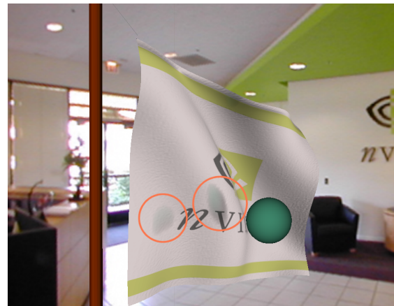
Dynamic cloth simulation with mesh deformation, bump mapping, and simple ray tracing. The vertex program displaces the flag's mesh away from the ball when contact would otherwise occur. The same program does bump mapping setup for the flag's surface. The program also computes a local reflection (circled in the image) of the green ball via ray casting. Written in DirectX 8. Credit: Doug Rogers.
