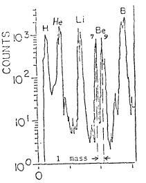
In this example graph, we see the number of data points for each elemental mass. In this graph, the standard chemical element abbreviations are used. The distance of one mass unit is indicated between beryllium-7 and beryllium-9.
