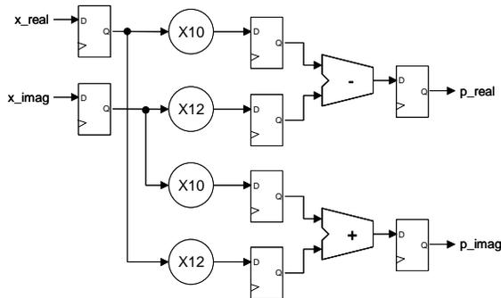
Figure 5. Circuit to multiply by  $10 + j12$
