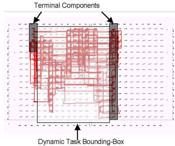
Figure 6. Post-APR layout of the  $10 + j12$  dynamic task. This comprises the four multipliers shown in fig. 5, surrounded by terminal components. The areas highlighted in gray indicate terminal components, while the area highlighted in white indicates the dynamic task bounding-box
