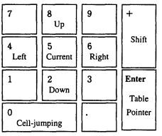
Figure 3: Key functions of the numeric keypad
