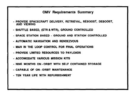
The OMV will provide several services to various types of spacecraft including new and existing satellites. The OMV can be controlled through the shuttle's payload interface, from the Ground Control Console at JSC, or from the Space Station. It has automatic navigation and rendezvous capabilitiy and does require man in the loop control for final operations such as docking with the Space Station or payloads.
