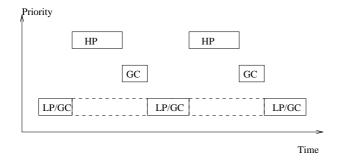
Figure 1: Dividing the CPU time between processes. The system consists of one periodic high priority process (HP) and one low priority process (LP). Whenever a high priority process is suspended, and no other HP process is eligible for execution, the garbage collector (GC) is run. GC work is also interleaved with the low priority process using traditional incremental garbage collection.
