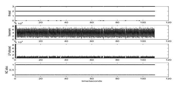
Figure 6: A run of the ball-on-beam system with log-data allocations made non-critical. In the thread plot you see that the UI thread gets CPU time throughout the run. The third plot shows the amount of memory allocated by low priority processes during this cycle. The fourth plot shows if non-critical allocations succeed or not; high level means success and low level is deny.
