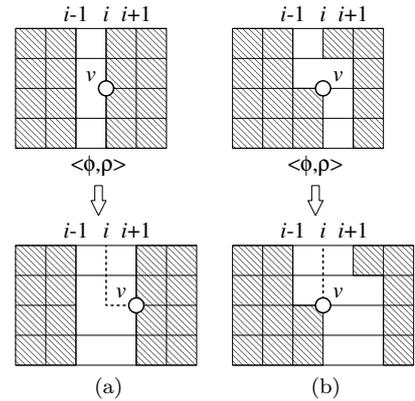
**Fig. 1** Layout with an exit track from  $v$  (represented by dotted lines) which is obtained from a layout  $\langle \phi, \rho \rangle$  by inserting an additional column. Figures (a) and (b) show the cases that the free edge  $e$  incident to  $\phi(v)$  is  $((i-1, j), (i, j))$  and that  $e = ((i, j), (i, j-1))$ , respectively.
