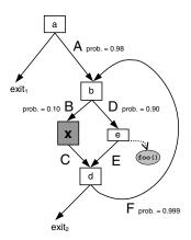
Figure 3: Control flow graph fragment with edge profile information. Block e calls subroutine foo().
