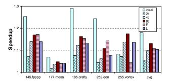
Figure 9: Limit study performance. "Perfect I\$" speedup if all I-accesses hit. "nt" prescient instruction prefetch speedup for n thread contexts. "F" spawn-target pairs selected assuming four thread contexts and fast helpers (low  $\mathrm{CPI}_h$ ), performance modeled so that helpers do not block on an I-cache miss. "L" 4t and spawn-target pairs selected with low reaching probability threshold (0.75).
