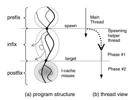
Figure 2: Prescient Instruction Prefetch. (a) Control-flow graph with spawn and target points highlighted. From profiling, the region labeled post-fix is known to encounter heavy instruction cache misses. (b) Two phases of helper thread execution: Phase #1 live-in precomputation; Phase #2 postfix precomputation and instruction prefetch.
