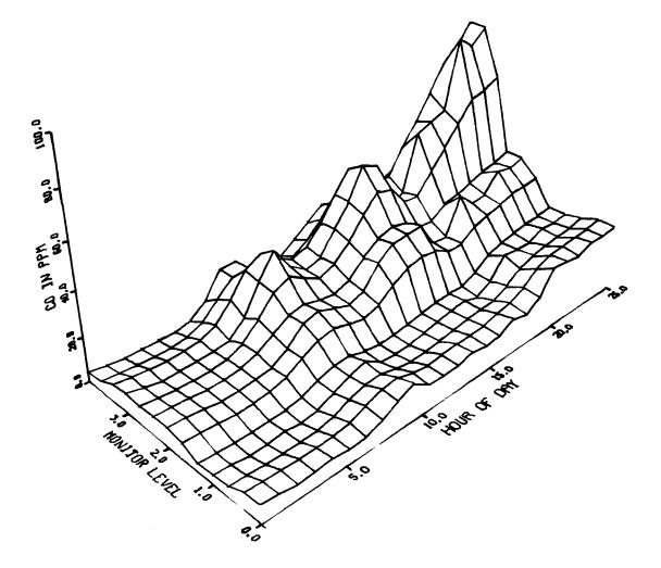
Figure 4. Carbon monoxide concentrations at 5 vertical locations over a 24-hour period for February 3, 1980, at the University of Minnesota Duluth Gasifier Facility.
