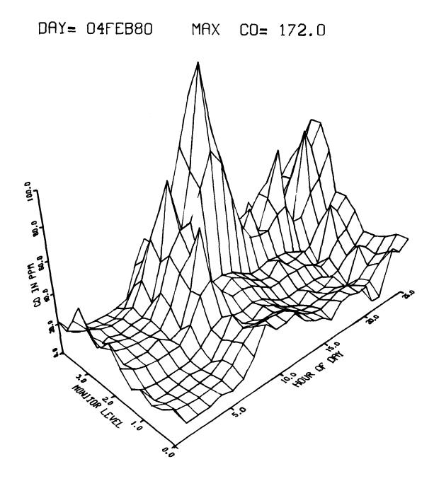
Figure 5. Carbon monoxide concentrations at 5 vertical locations over a 24-hour period for February 4, 1980, at the University of Minnesota Duluth Gasifier Facility.
