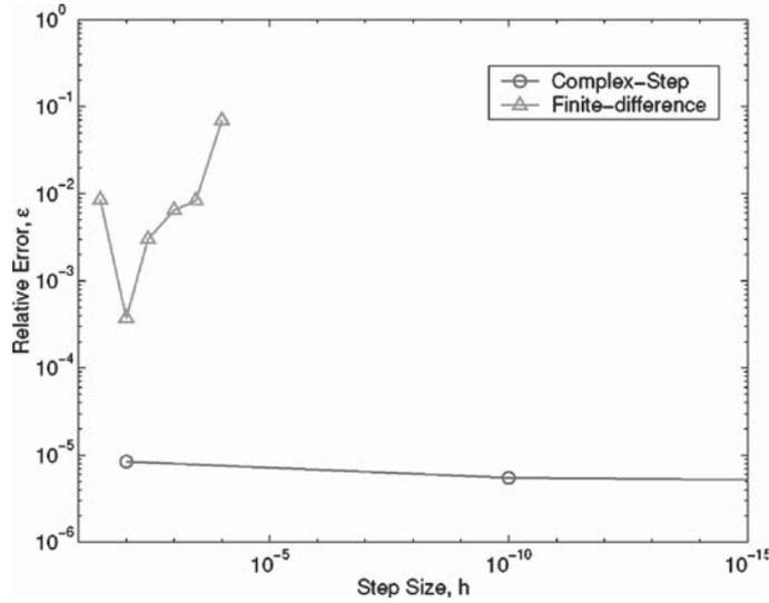
Fig. 4. Sensitivity estimate errors for  $\partial C_D / \partial b_1$  given by finite-difference and the complex step for different step sizes;  $\varepsilon = (|f - f_{ref}|) / |f_{ref}|$ ; reference is complex-step estimate at  $h = 10^{-20}$ .
