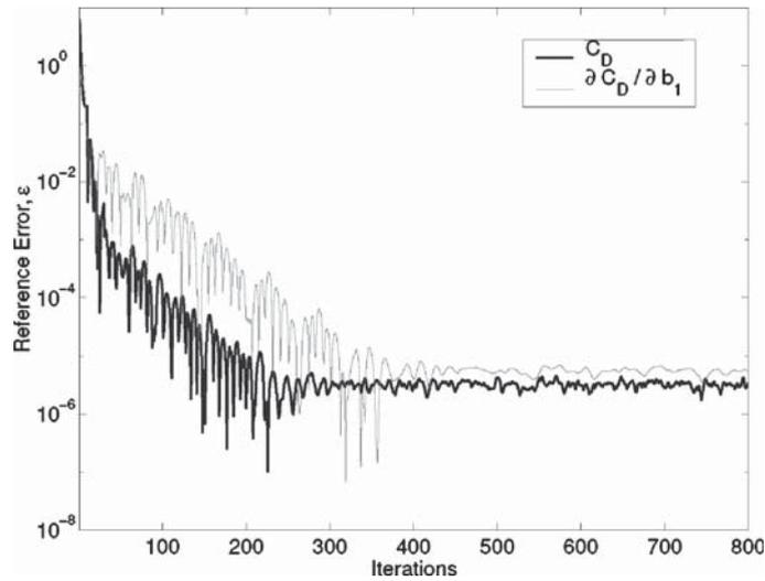
Fig. 3. Convergence of  $C_D$  and  $\partial C_D/\partial b_1$  for the 3D aero-structural solver;  $\varepsilon = (|f - f_{ref}|)/|f_{ref}|$ ; reference values from the 801st iteration.
