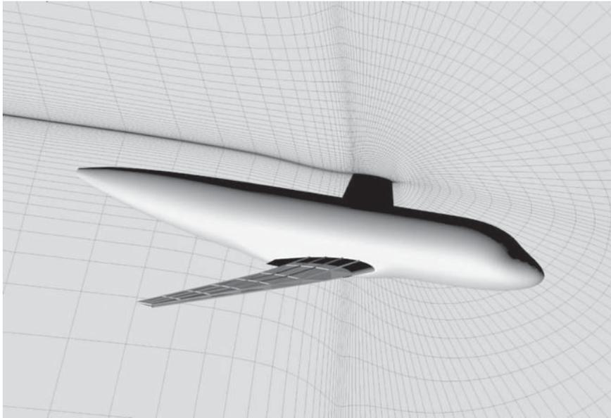
Fig. 2. Aero-structural model and solution of a transonic jet configuration, showing a slice of the grid and the internal structure of the wing.
