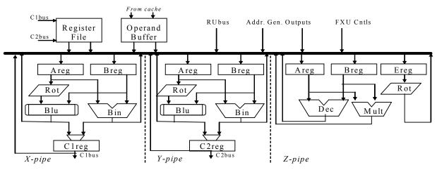
Figure 1. Block Diagram for the FXU dataflow stack.
