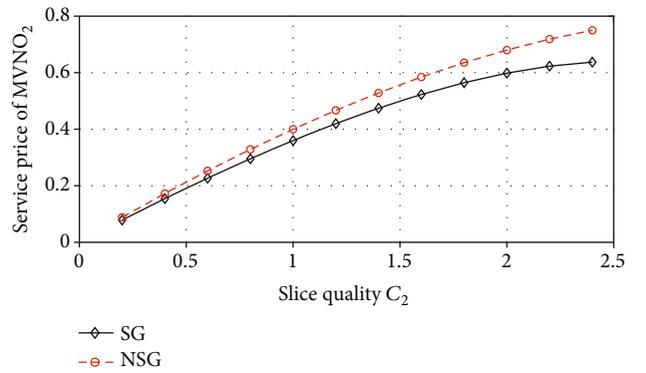
FIGURE 6: The equilibrium network price of MVNO<sub>2</sub> versus slice quality  $C_2$  in two cases.
