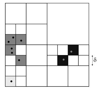
Figure 2: Contact Clustering Using Quadtrees. The contacts are represented by dots. Different intensities are used to highlight the different clusters. Octrees are used instead of quadtrees in our 3D implementation.
