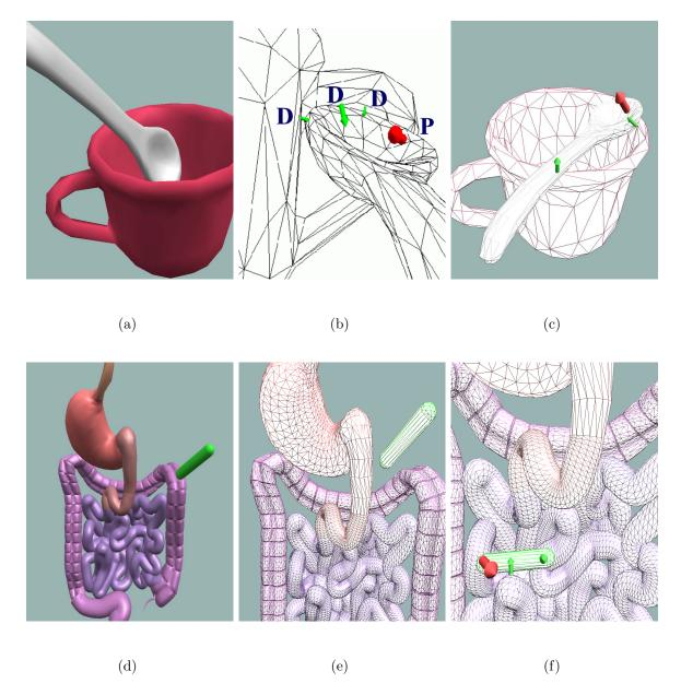
Figure 9: Two Contact Scenarios: a Cup interacting with a Spoon (Top) and Virtual Exploration of a Digestive System Model (Bottom). Figures in (b), (c), (e) and (f) show the forces computed at clustered contacts, for both disjoint (D, green arrows) and penetrating (P, red arrow) situations.
