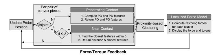
Figure 1: Haptic Display Pipeline
