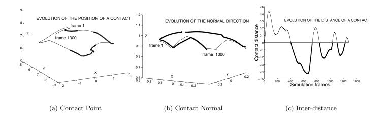
Figure 12: Contact Profile for a Single Contact Scenario. The thick solid line represents that the objects inter-penetrate, and the thin solid line indicates that the objects are disjoint. Notice the smoothness of the contact data.
