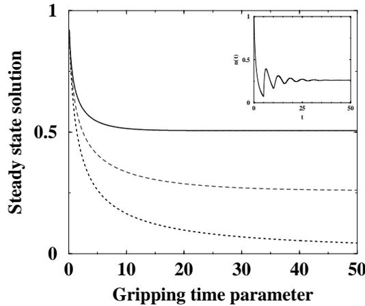
Figure 7. Steady-state solution versus (dimensionless) gripping time parameter  $\tau$ : for  $\beta = 0.5$  (short dash), 1 (long dash), 1.5 (solid line). Inset shows a typical relaxation to the steady state for  $\tau = 5, \beta = 0.5$ .
