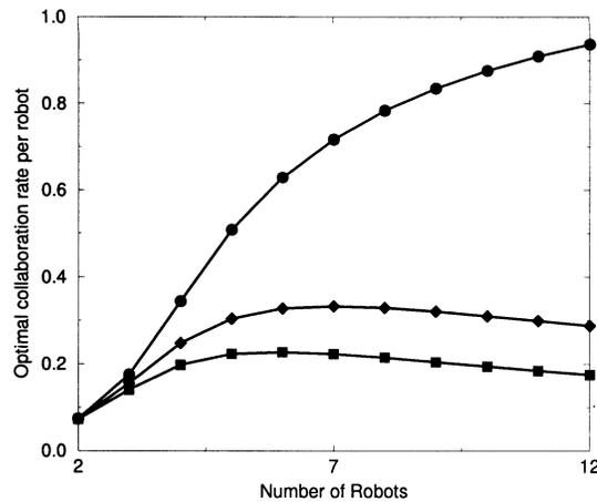
Figure 9. Relative collaboration rate versus the number of robots for different values of interference strength:  $\tau_{av} = 0$  (circles),  $\tau_{av} = 0.5$  (diamonds), and  $\tau_{av} = 1.0$  (squares).
