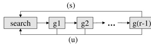
Figure 2. Macroscopic state diagram of collaboration in a multirobot system. The arrow marked “s” corresponds to the transition to the search state after a successful collaboration has occurred, while the arrow marked “u” corresponds to the transition after an unsuccessful collaboration, that is, when waiting time exceeded  $\tau$ .
