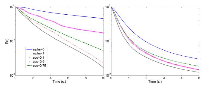
Figure 3: Average of functions E(t) for MU using different values of  $\epsilon$ , with  $\alpha = 0$  and  $\alpha = 1$  for reference (see Section 3.1): (left) dense matrices, (right) sparse matrices. Same settings as in Figure 1.
