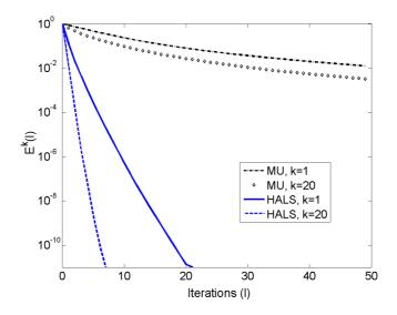
Figure 7: Evolution of the relative error  $E^k(l)$  of the iterates of inner iterations in MU and HALS, solving the NNLS subproblem  $\min_{W\geq 0} ||M - WH^{(k)}||_F$  with r = 40 for the classic text dataset (cf. Table 2).
