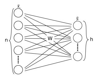
Figure 1: Schematic illustration of the network: an input  $\vec{x}_{\nu}$  is fed to an input layer of n neurons, connected to h neurons that produce the output  $\vec{y}_{\nu}$ . The weight matrix W contains also the thresholds that appear as weights of a fictitious 0-th input clamped at 1.
