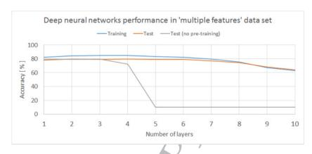
Figure 8: Results of deep neural networks on the multiple features data set. Without pretraining, after layer 5, the accuracy drops to the baseline of 10%, or what could be expected from a model choosing at random.
