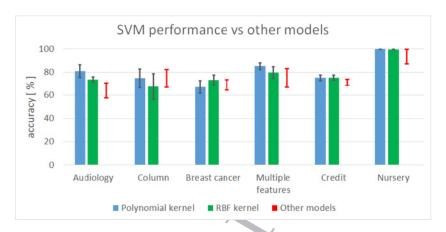
Figure 7: SVM models (with polynomial and RBF kernels) compared to the rest of the models introduced in Figure 2. The red interval represents the range (minimum and maximum) of the accuracies of the eight other models. In four out of the six sets, kernel machines surpass the maximum obtained by these previous classification algorithms.
