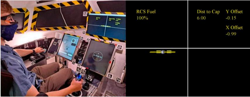
Figure 1. Experiment Environment and Primary Display. *Note.* Example participant seating, hand positioning, and displays during a trial are shown at left, and an enlarged example of the primary display is shown at right. On the primary display the virtual space station, camera crosshairs, offset indicators, reaction control system (RCS) fuel indicator, and distance (“Dist”) to capture (“Cap”) indicator can be seen. See Figure 2 for enlarged examples of the secondary display.
