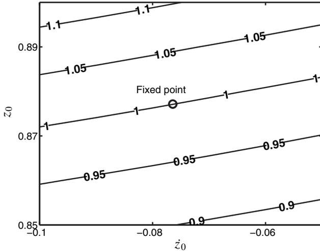
Fig. 4. Contour plot of  $|\det(D_x R(\bar{x}))|$  for the leg angle trajectory (49) with  $k = 1$ . The fixed point  $\bar{x} \approx (0.8772, -0.0764)^T$  lies on the  $|\det(D_x R(x))| = 1$  contour, whereas volume (area) is not preserved away from the fixed point.
