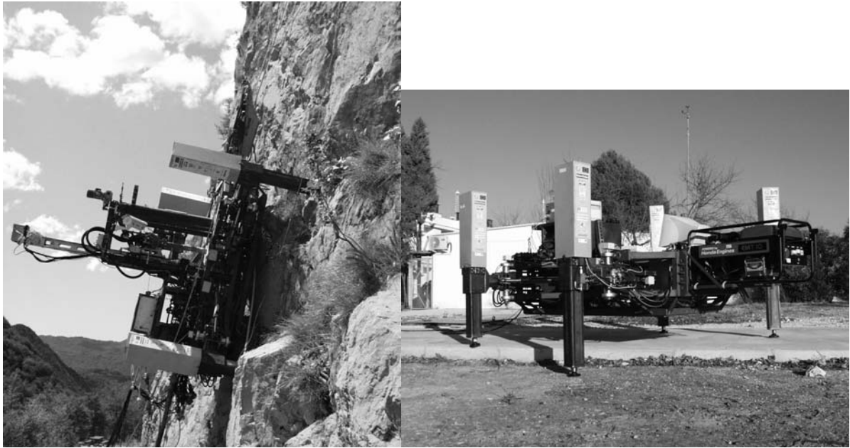
Fig. 3. ROBOCLIMBER field tests: a) Climbing: Alps, Northern Italy; b) Walking: Industrial Automation Institute (IAI-CSIC) outdoor facilities.
