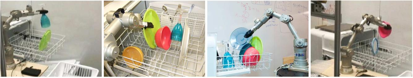
Figure 14: Dishwasher experiments (Section 6.3): Our robotic arm unloads items from a dishwasher.
