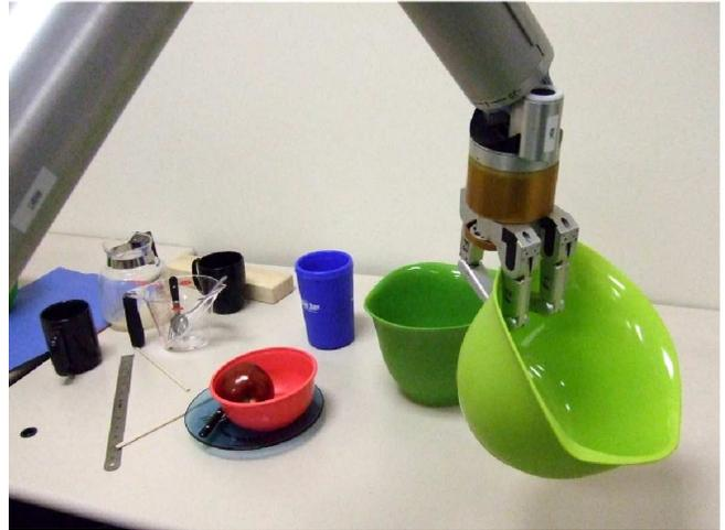
Figure 17: Barrett arm grasping an object using our algorithm.
