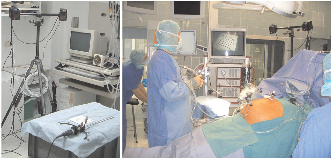
Fig. 6. Left: optical tracking system smARTtrack1 in the laboratory and right: smARTtrack1 in the operating room during an endoscopic surgery (images courtesy of F. Vogt).
