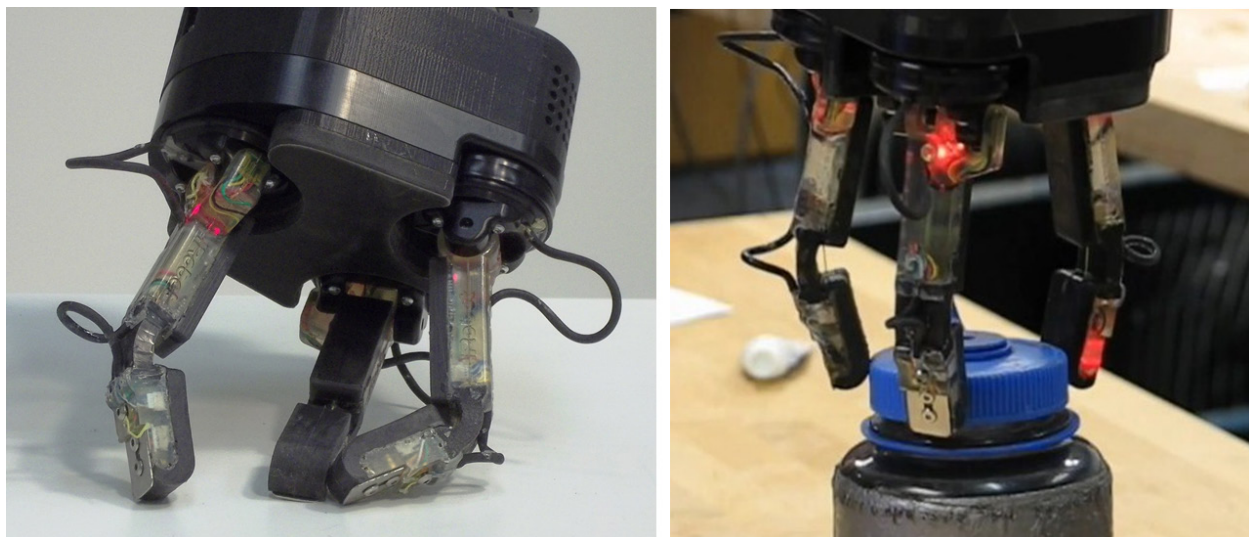
Fig. 18. Compliance during tasks; fingers deform during unintentional contact with a surface (left), and passive adjustment of the fingers during lid tightening task (right).
