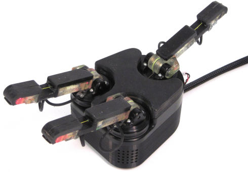
Fig. 1.i-HY is an underactuated hand capable of performing a wide range of tasks, including fingertip grasping and manipulation.
