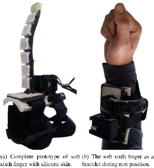
Figure 8. The complete prototype of the soft sixth finger with silicone skin. The device can be worn on the arm using elastic band. It can be shaped as bracelet when being not used to reduce the encumbrance of the device.
