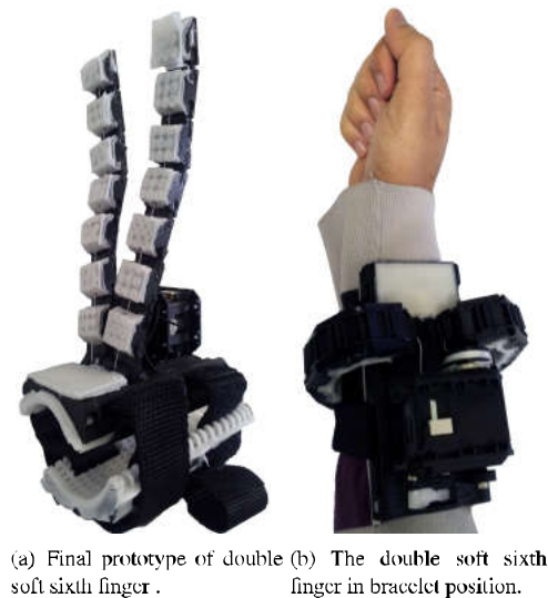
Figure 12. The final prototype of double soft sixth finger, the device can be worn on the paretic arm through support base and elastic straps. It can be shaped into bracelet when being not used.
