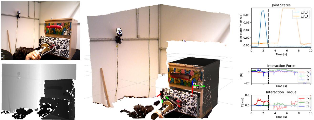
**Figure 3.** Visualization of the sensor data for opening a drawer: RGB and depth image (*left*), mesh model, point cloud and coordinate frames of tracked bodies (*middle*), and drawer state and applied wrenches (*right*) with dashed vertical line indicating current time.
