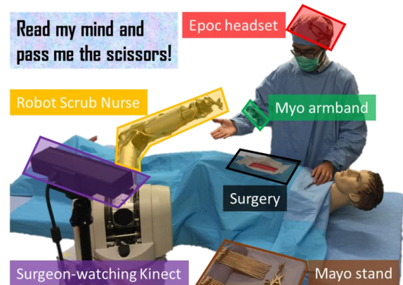
Figure 2. Illustration of a RSN system. Various sensors (Kinect, Epoc and Myo) are used to capture human’s communication cues, which are fed into the TTSNet framework for turn-taking analysis. The network output are precise inferences about the delivery of surgical instruments ahead of time.
