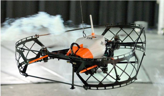
Figure 4. Experimental verification of the presented methods is done by flying a coaxial hexacopter in a 3D wind tunnel. The hexacopter hovers autonomously using a position controller, based on pose measurements from an external tracking system. For comparison, we also log data from a stereo vision based onboard pose estimator. The figure shows flow visualization at a wind velocity of around 6 m/s. We loosely suspended the robot on a filament for safety purposes.
