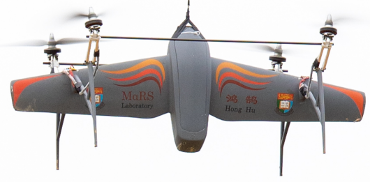
Fig. 7. Our quadrotor tail-sitter UAV prototype: Hong Hu.
