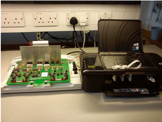
Figure 10. Printer and ELVIS and ELVIS Power Interface Daughter Boards.
