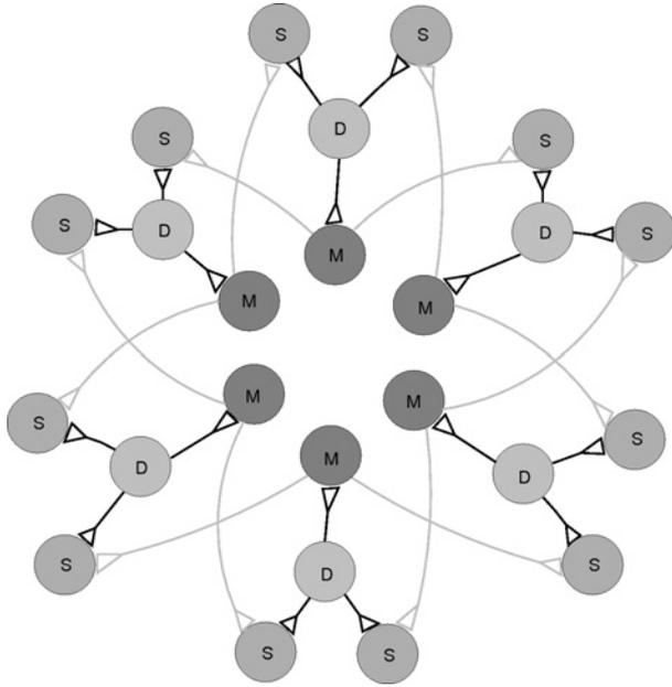
**Figure 6** A network with six direction cells. Motors and the recurrent of memory neurons were not drawn. Each sigmoid neuron is connected to either a left or a right turn motor.
