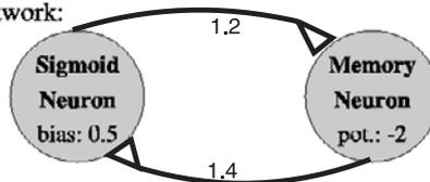
**Figure 2** Marker-Based Genetic Encoding: a chromosome consisting of integers is interpreted as a neural network. A start marker is any number that modulo  $k$  results in a remainder of 1 and an end marker is any number that modulo  $k$  results in a remainder of 2.  $k$  is typically chosen somewhere between 5 and 15.
