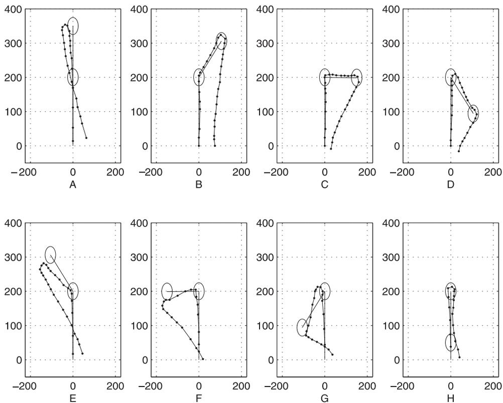
**Figure 9** Robot path integration experiments. The home (starting) position of the robot is at (0,0) for all experiments. The positions of the waypoints are highlighted with circles. The mean error over these runs was 46.625 cm with a standard deviation of 18 cm. (A) 69 cm; (B) 75 cm; (C) 31 cm; (D) 43 cm; (E) 51 cm; (F) 21 cm; (G) 41 cm; (H) 42 cm.
