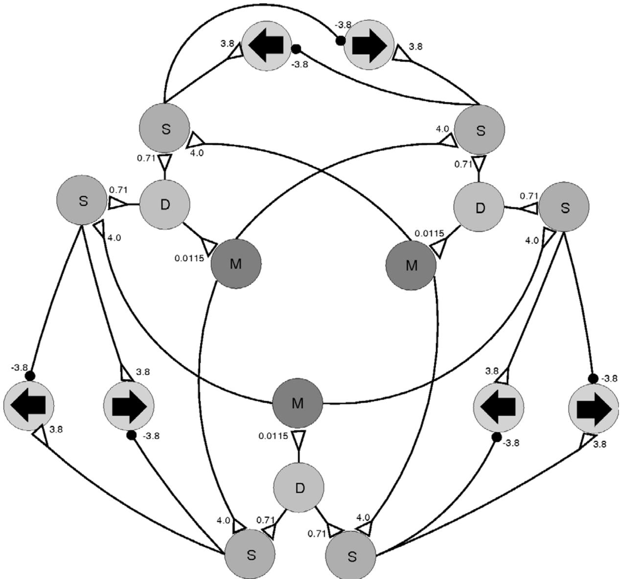
**Figure 3** Evolved network using direction (D) cells. Each direction cell has one memory (M) CTRNN cell and two sigmoid (S) neurons associated with it. For illustration purposes, the turn motors (represented by the left and right arrows) are duplicated and the recurrent connections of the memory neurons onto themselves are omitted.
