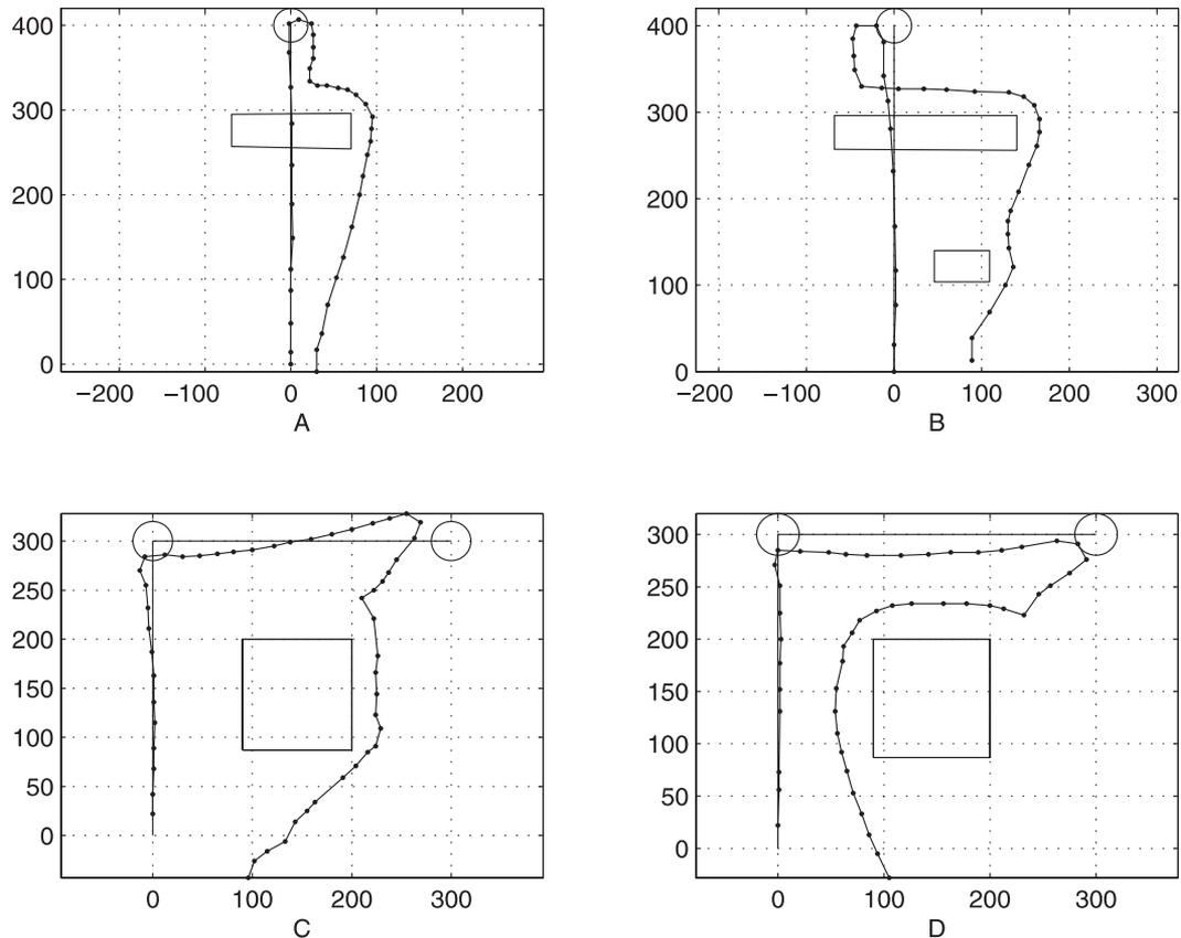
**Figure 12** Robot path integration and obstacle avoidance experiments. The obstacles were only placed into the arena after the agent reached the last waypoint and started its homeward journey. The errors were (A) 32 cm; (B) 92 cm; (C) 105 cm; and (D) 108 cm.
