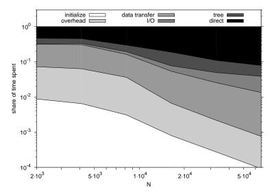
Fig. 3. Relative cumulative share of time spent by the living simulation tasks as a function of the number of simulated particles. From top to bottom the areas refer to the share of time spent on direct integration, tree integration, local file I/O, grid data transfer, grid job submissions and simulation initializations. Note that both axes are in log-scale.
