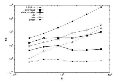
Fig. 2. Timing measurements of the living simulation tasks as a function of the number of simulated particles. The two solid lines represent time spent on direct integration (bullets) and tree integration (circles). The thick dashed lines indicate grid overhead by data transfers (open squares) and job submissions (filled squares). Finally, the two thin dashed lines indicate overhead caused by local file I/O (open triangles) and code initializations (filled triangles).
