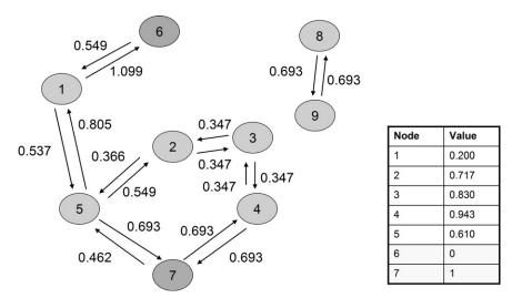
**Figure 1.** The network constructed based on the example in Table 1. Nodes 1 through 5 are unknown nodes, and nodes 6 and 7 are preassigned nodes. Nodes 8 and 9 are removed from the network because they fall outside the transitive closure of the preassigned nodes.
