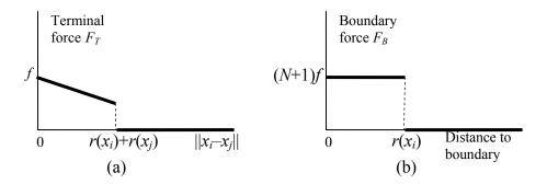
FIGURE 3 Possible definitions of forces: (a) repulsive force for terminal pair (*i*, *j*); (b) boundary force for terminal *i*.
