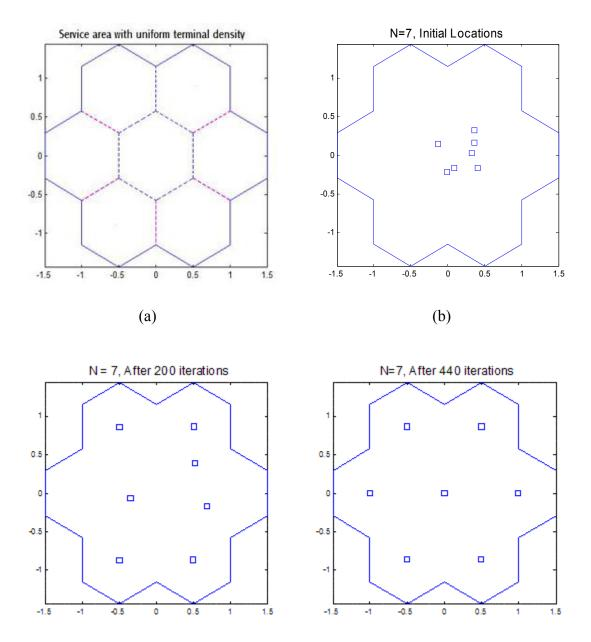
FIGURE 4 Verification of convergence: (a) area *S*; (b) initial locations; (c) locations after 200 iterations; (d) equilibrium locations after 440 iterations.
