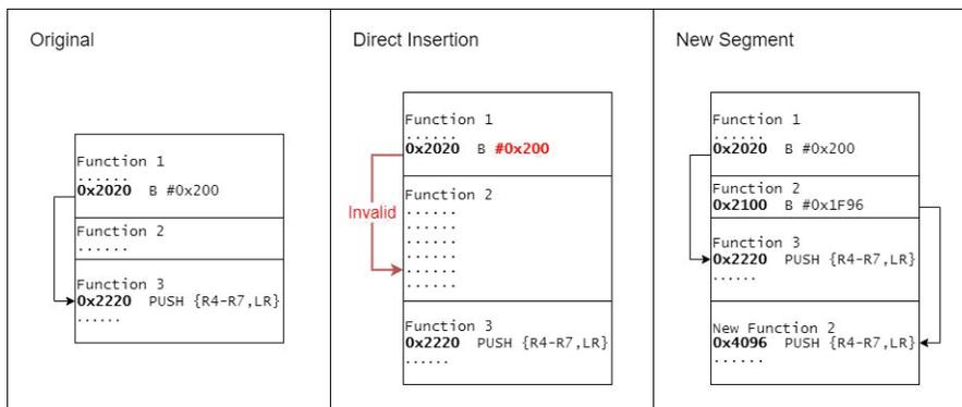
**Figure 4** Direct Insertion vs New Segment procedures.
