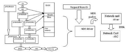
Figure 3 Basic principle of reading and send the memory contents
