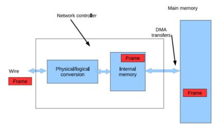
Figure 1 Ilustration of how DMA is used when network driver communicates with the network card (NIC) [13]
