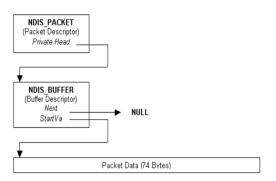
Figure 2 A simple version of NDIS buffer chaining [15]
