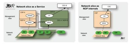
Figure 4 Management models for network slicing.
