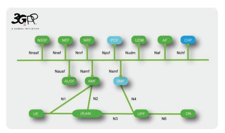
Figure 6 New charging function (CHF) and service based interface Nchf.
