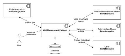
Figure 4 The scheme for the WUI measurement platform.
