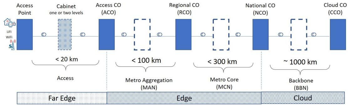
Fig. 1. High-level network architecture
