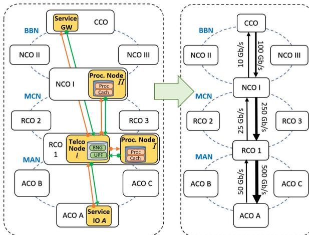
Fig. 4. Example of mapping service into network traffic
