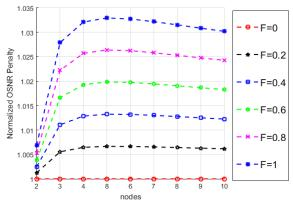
Fig. 13. Normalized OSNR Penalties against Different Fiber Switch Requests and Hops (F=0 as reference)
