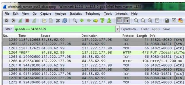
Fig. 9: Control messages at restful server level for bit rate change.
