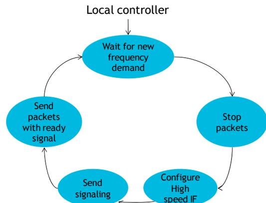
Fig. 4: Finite State Machine for hitless behaviour.
