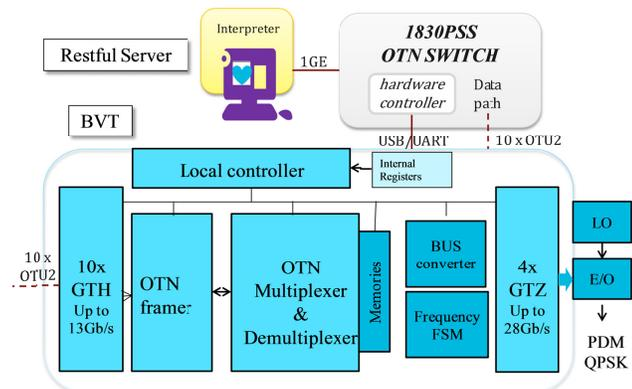
Fig. 2: Architecture of Elastic Optical Interface with controller
