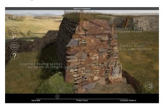
Figure 2: The cut-away reconstruction of the wall at Castle Law Forgandenny.
