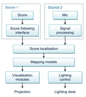
Figure 1: Overall system architecture
