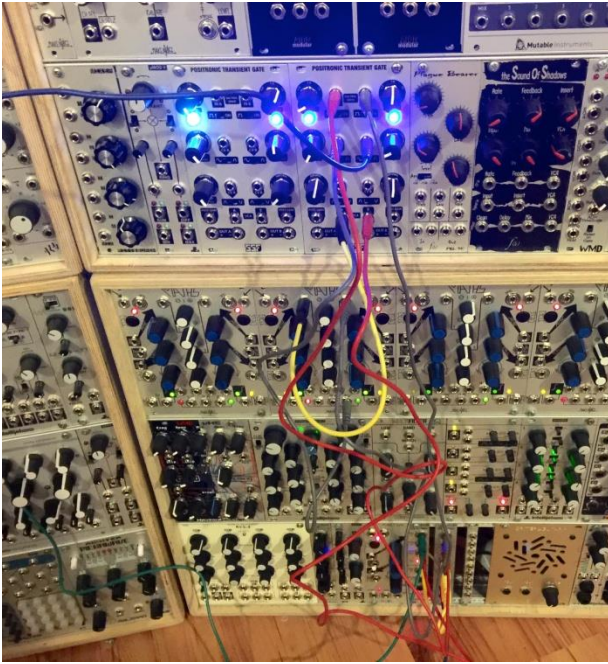
Figure 4. The implementation of the logistic equation on the Eurorack synthesizer.
