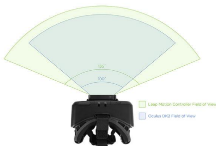
Figure 10: Oculus Rift HMD FOV and Leap Motion Controller FOV
