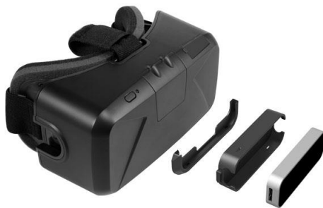
Figure 9: Oculus Rift Head-mounted Display with Leap Motion Controller Integration
