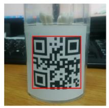
Figure 7 Recognition test of QR code on cylinder type object (see online version for colours)
