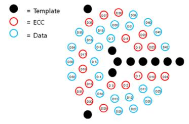
We set the centred line as a template for projective transformation correction. There are centred point and sine and cosine cost is zero of each circle. Templates help in detecting and recognising image rotation and in determining the skew from the camera
