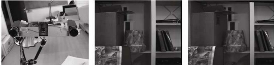
Figure 3 The Time-Of-Flight stereo rig and the rectified image pair I_l and I_r used in the experiment
