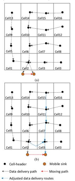
When the mobile sink moves to Cell 3, the cell-header in Cell 3 becomes a new OCH and execute Rule 2 to update the routes from downstream cell-headers to the current OCH. The downstream cell-header means cell-headers, i.e., 7, 11 and 15. Furthermore, the current cell-header executes Rule 3 to update the routes from the previous OCH to the current OCH. Blue arrows represent adjusted data delivery routes. The specific algorithm is also shown in Algorithm 1.
