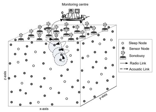
Figure 1 Multi-sink network architecture for IoUTs
